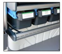
Lashing strap with clamping lock and ProSafe hook.
